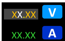
Voltage (V) setting selected and the 'units' digit being edited.
